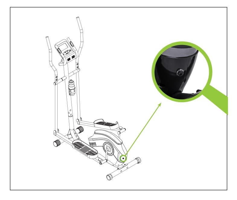
The adapter connection is located on the back of the device (see illustration). Attach the adapter to the adapter connection and connect to the power supply. You can now use the elliptical trainer.
