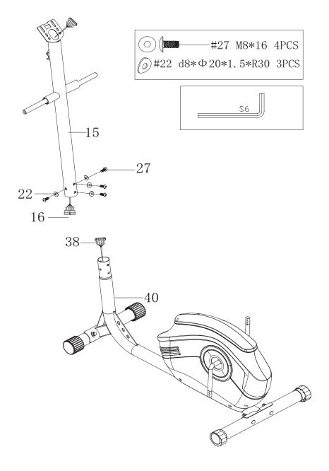
Connect the Sensor 16 and 38, fix the Upright Post (15) with the Main Frame (40) with Nut (27)
